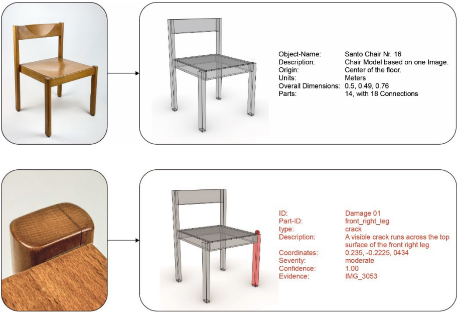
Figure 32: Generation of an assembly-model from a single reference image and user comments (top), as well as damage detection and annotation, linking a visible crack on the front right leg to structured metadata (bottom).
