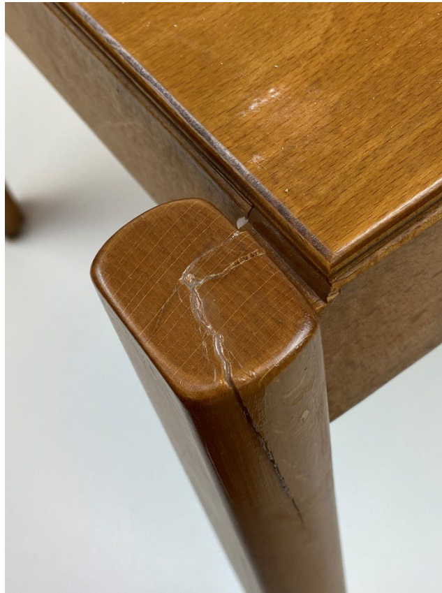
Figure 39: Previous attempt of a repair on chair 5.
