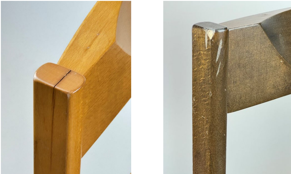
Figure 34: Typical damages of the chairs: Cracking on the legs (left) and chippings and scuff marks (right).
